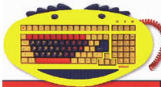
Figure 1. KidBoard, a color-coded computer keyboard for children. Keys that should be pressed with the left hand are colored differently than the right-hand ones. Moreover, each key also has a tiny picture of an object whose name begins with that letter (a - apple, etc.). Reproduced with permission from http://www.webchild.com/kidboard.htm
